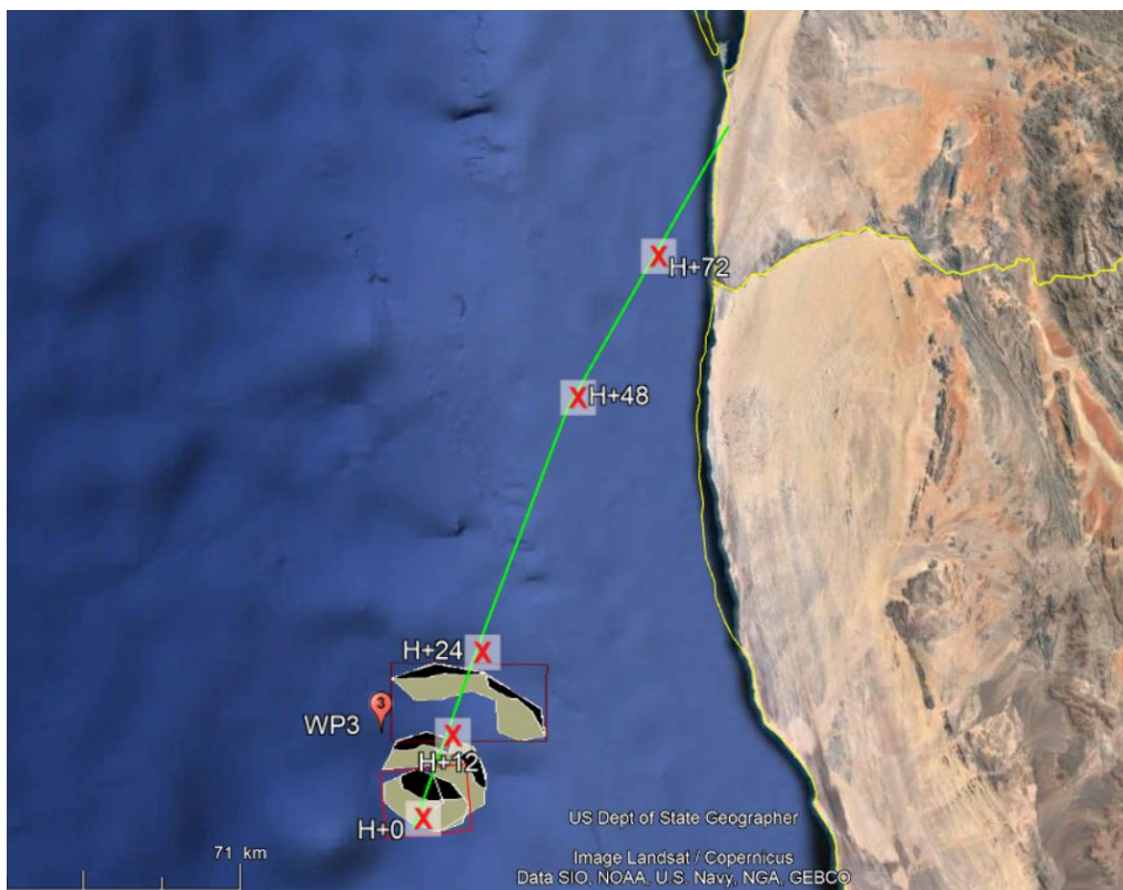
Figure: oil trajectory (green line and time markers) according to the metocean conditions provided for the exercise and results of aerial surveillance provided to the participants in injects 4, 7 and 9.
